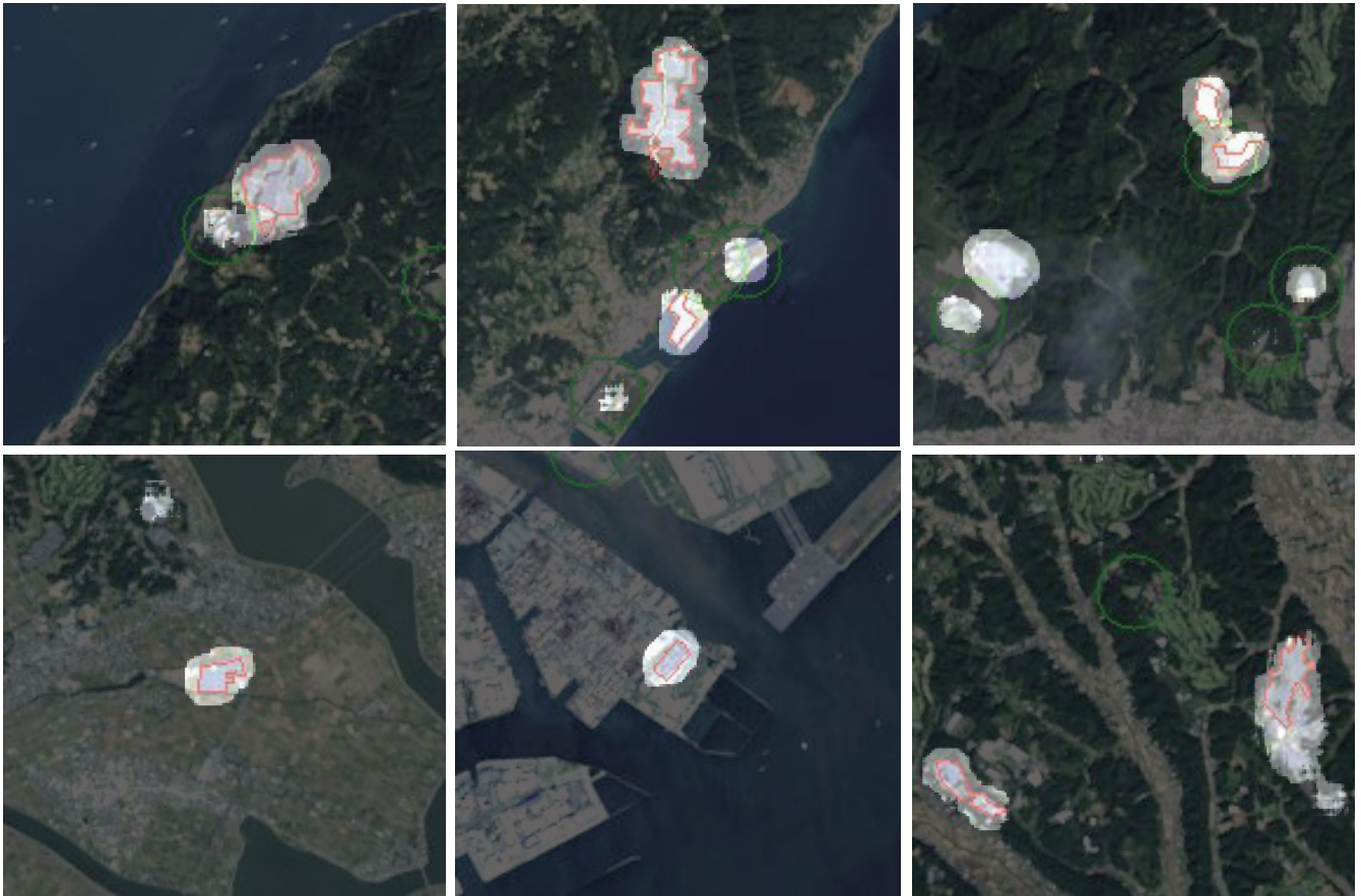
Fig. 7: Detection results for our approach. Detection regions are highlighted. The solar power plants with more than 5MW output are enclosed by red polygons, while the smaller powerplants are denoted by a green circle with a radius of 480m.
