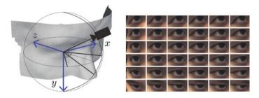
Fig. 8.7 Training data synthesis. *Left* Placement of the virtual cameras. *Right* Examples of synthesized eye images (Reproduced with permission of © 2014 IEEE [45])
