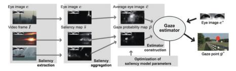
**Fig. 8.4** Illustration of the saliency-based calibration approach. The method consists of mainly four steps: saliency extraction, saliency aggregation, estimator construction and saliency model optimization (Reproduced with permission of © 2013 IEEE [44])
