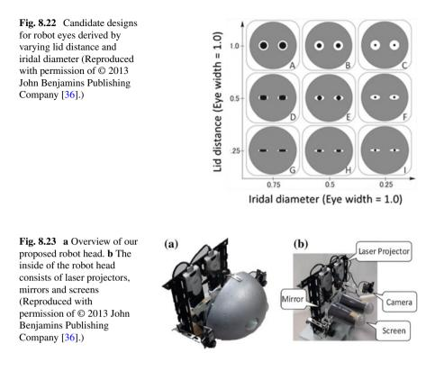
iris diameter. In addition, by replacing the mask, we can change the outline shape of the eyes.
