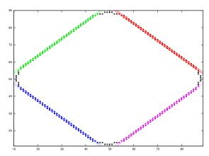
Figure 13. Digital line recognition by our method
