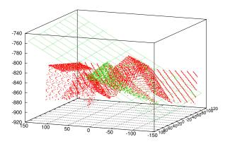
Figure 12. Digital plane recognition for 3D real data by our method
