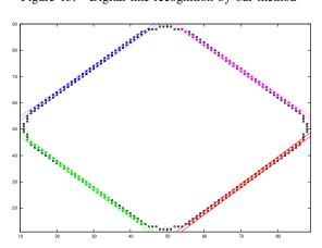
Figure 14. Digital line recognition by RANSAC
