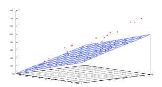
Figure 9. An example of 3D synthetic data and a recognized plane by our method (red: outliers, blue: digital plane)
