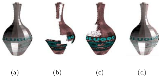
Fig. 7 Simulation with two light sources. (a) input image; (b) our albedo image in non-ambiguous regions; (c) our obtained albedo image; (d) albedo image using the diffuse reflection model.
